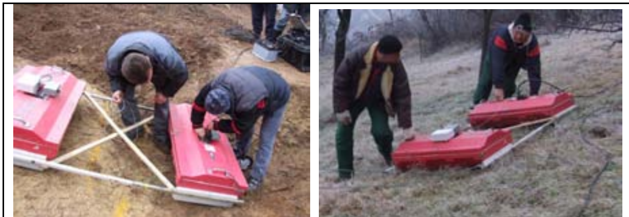
figure 2: radar antenna 100 kHz
