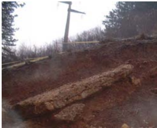
figure 66: The electricity cable doped to the measuring area. The high voltage influenced the 100 MHz radar measurement.
