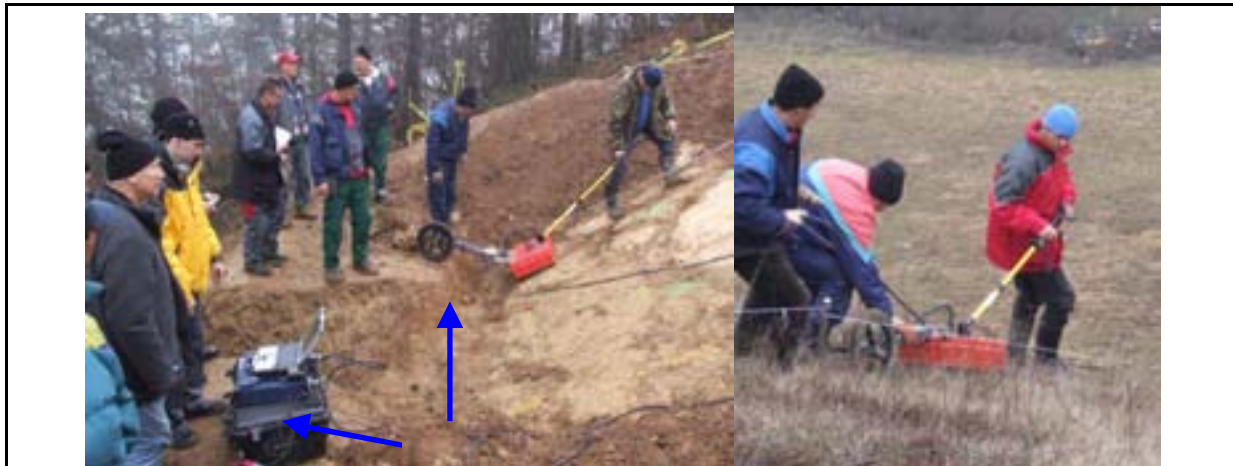
figure 1: radar equipment left: computer, middle and right: radar antenna 270 kHz
